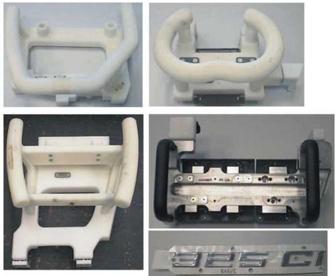
Figure 4: Four devices for attaching the model badge at the rear of the vehicle
